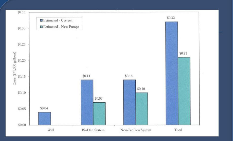
Power Cost at Coyle Denitrification Plant Unit electric power cost: \$0.0532/kwh
