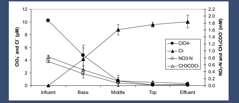
$ClO_4^-$ ,  $NO_3^-$ ,  $CH_3COO^-$ , and  $Cl^-$  concentration profiles in the biofilm reactor receiving 10 mg.L<sup>-1</sup>  $NO_3^-$ N and 1,000 µg.L<sup>-1</sup>  $ClO_4^-$ , and 42 mg.L<sup>-1</sup>  $CH_3COO^-$ .
