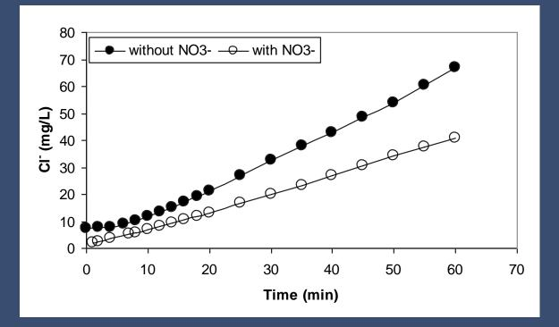
Effect of 2 mM (28 mg/L) nitrate-N on reduction of 2 mM (200 mg/L) perchlorate in flasks inoculated with perchlorate-reducing culture, average MLSS in flasks was 5 g.L<sup>-1</sup>. 16.7 mM acetate was added to both flasks. C:(ClO<sub>4</sub>+N)>1.8
