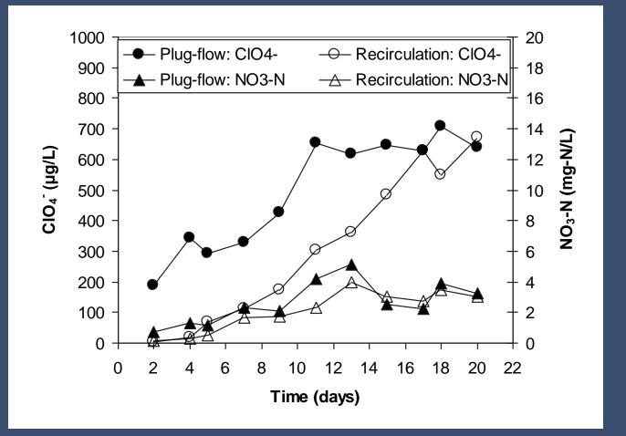
Influent contained 1,000  $\mu$ g.L<sup>-1</sup> ClO<sub>4</sub>, 16 mg.L<sup>-1</sup> NO<sub>3</sub>-N and 52 mg.L<sup>-1</sup> acetate.
