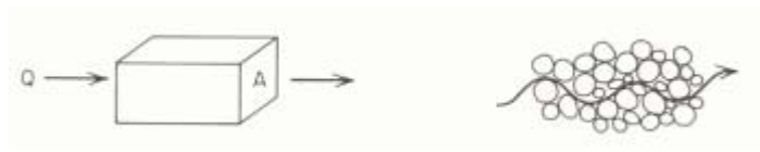
Figure 24. Macroscopic and microscopic concepts of porous medium flow (Freeze/Cherry, Groundwater, © 1979. Electronically reproduced by permission of Pearson Education, Inc., Upper Saddle River, New Jersey).
