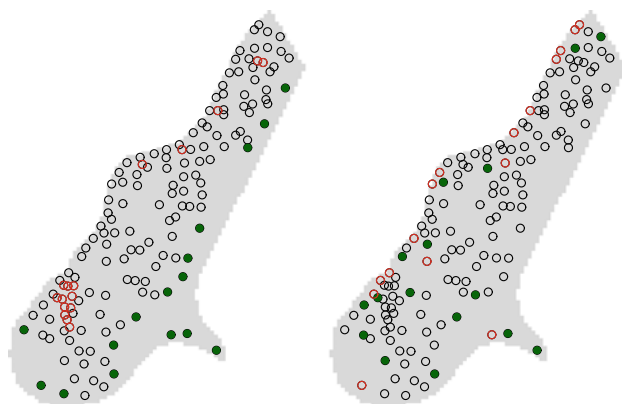
Fig. 8.16 Candidate points for removal. Left : for mean kriging variance, right : for delineating the 1,000 ppm contour. Open, red circles : 10 % most favourite points; closed, green circles : 10 % least favourite points
