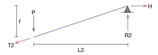
This is called portion '2'. It has horizontal extent L2. There are two reactions at the support. The vertical reaction is R2. The horizontal reaction is H. Cable tension is T2. H is equal to the horizontal component of T2.
