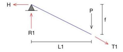
This is called portion '1'. It has horizontal extent L1. There are two reactions at the support. The vertical reaction is R1. The horizontal reaction is H. Cable tension is T1. H is equal to the horizontal component of T1.
