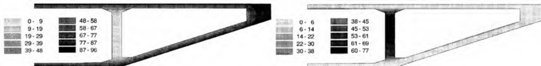
Figure 3.216: ASR extent percent and longitudinal plastic strains in box girder; Ulm et al. (2000)
