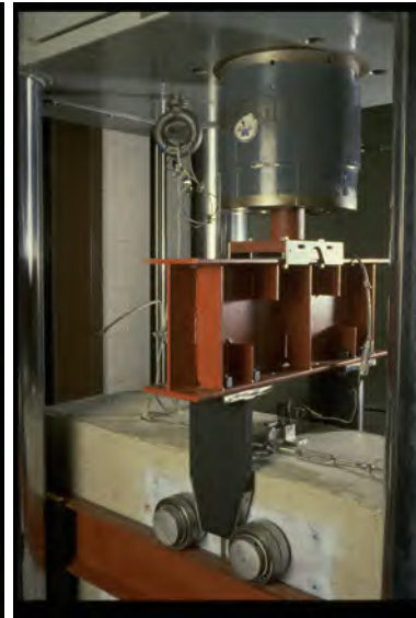
(b) Detail of the load application
