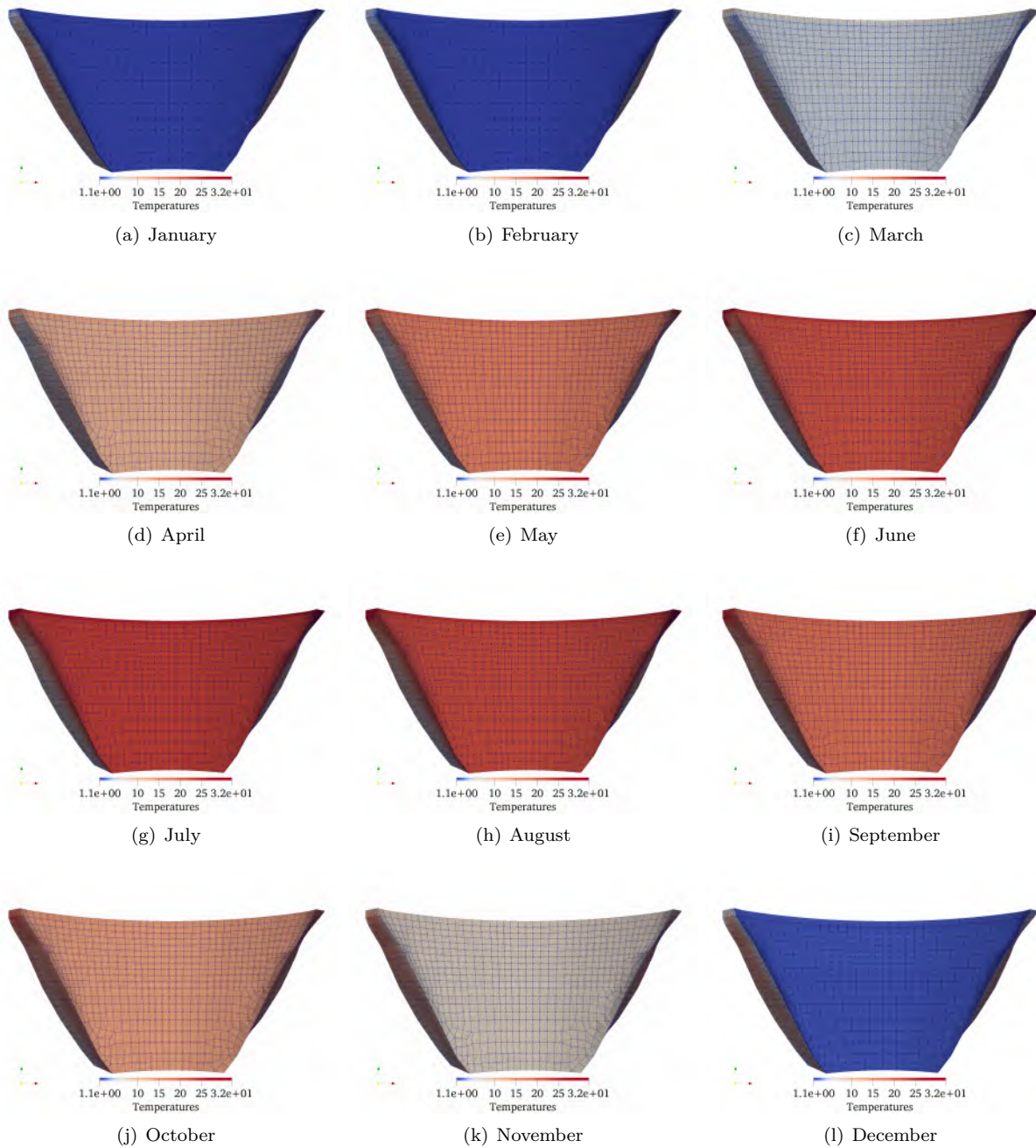
Figure 6.9: Temperature contour plots of various months throughout one year at the downstream face of
