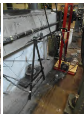
(c) Instrumentation; LVDT
