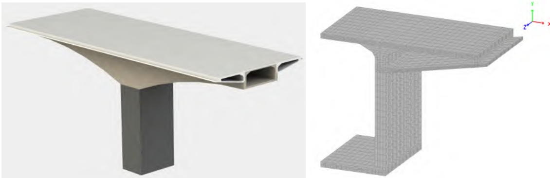
Figure 15.4: Finite element mesh
