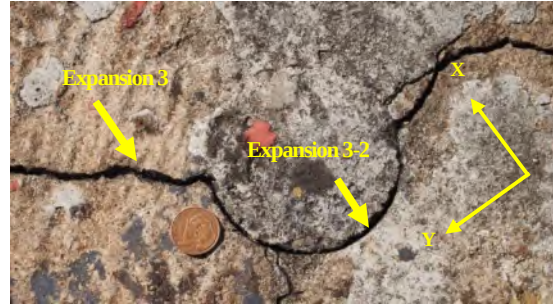
(b) Continued expansion around previous borehole. Adapted from Katayama (2017).
