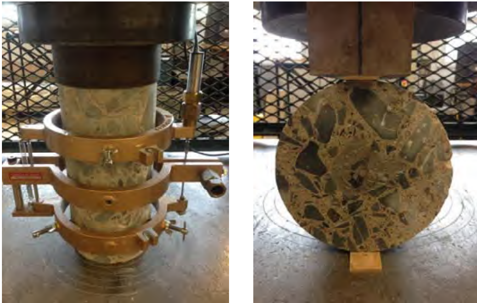
Figure 2.4: Modulus of elasticity, ASTM C469; and splitting tensile strength, ASTM C496
