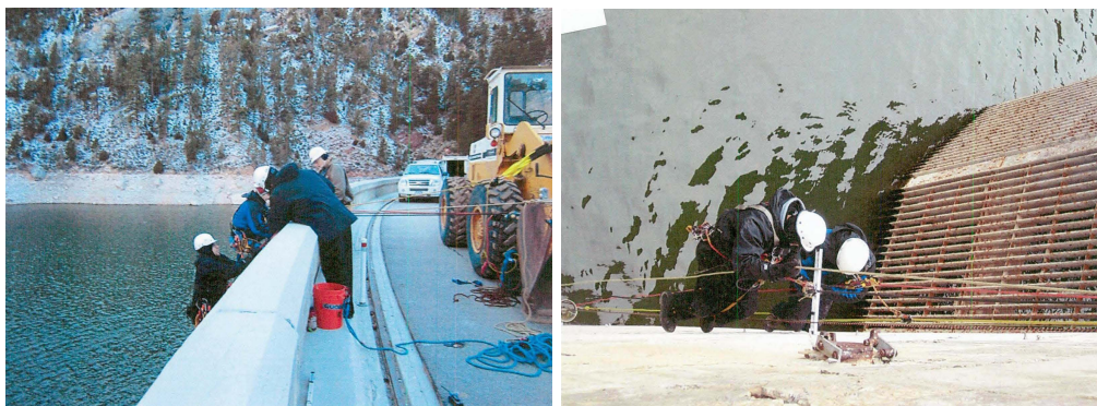
Figure A.4: Climb Team members measuring upstream dam face to plumb line (Lung, 2012)
