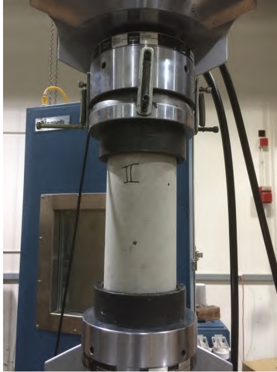
Figure 112 - Cylinder installed in MTS machine
