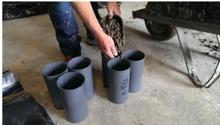
Figure 65 - Filling compression test cylinder molds
