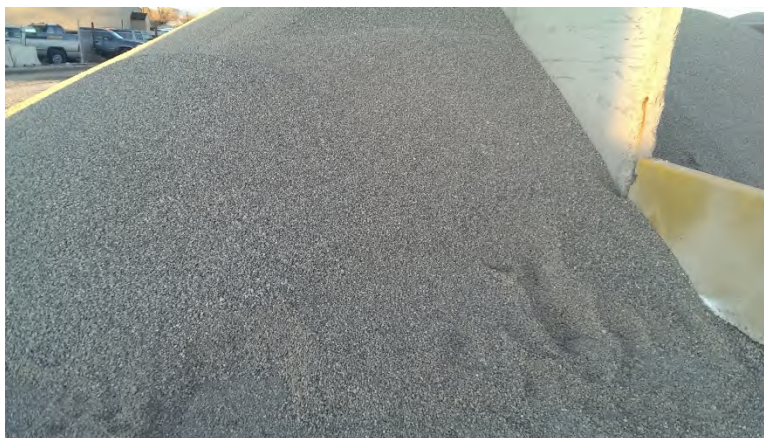
Figure 4 - 3/8" Gravel storage bin at Grand Junction Ready Mix
