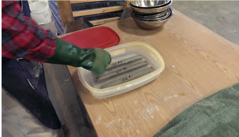
Figure 19 - After zero readings, bars were placed in 1N aqueous NaOH.
