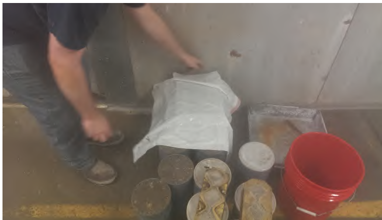
Figure 16 - Mortar bars placed in curing room and covered with plastic
