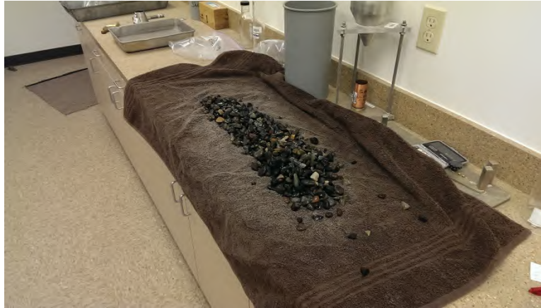
Figure 29 - Soaked coarse aggregate is spread on a towel for drying to saturated surface-dry condition.
