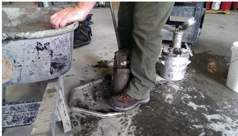
Figure 58 – The slump mold is filled in three layers, each tamped 25 times.
