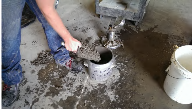
Figure 61 – The air meter bowl is filled in two layers, each rodded 25 times.
