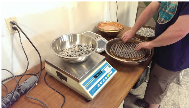
Figure 42 - Cleaning a screen during coarse aggregate sieve analysis
