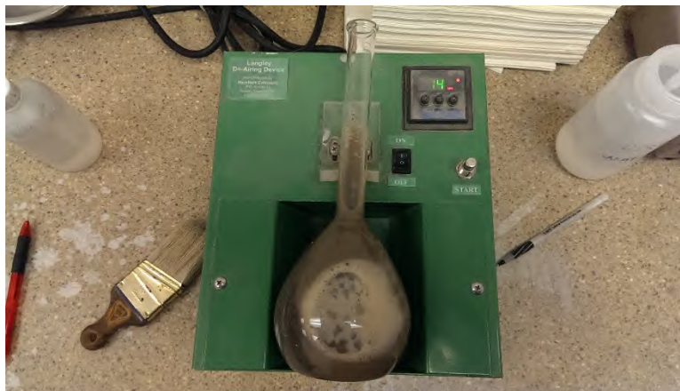
Figure 37 - The volumetric flask is rotated to remove trapped air.
