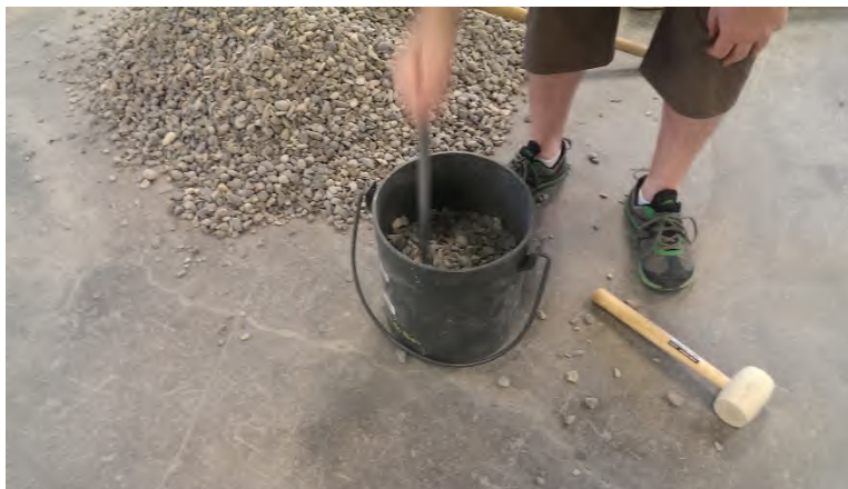
Figure 39 - Each lift is rodded 25 times.
