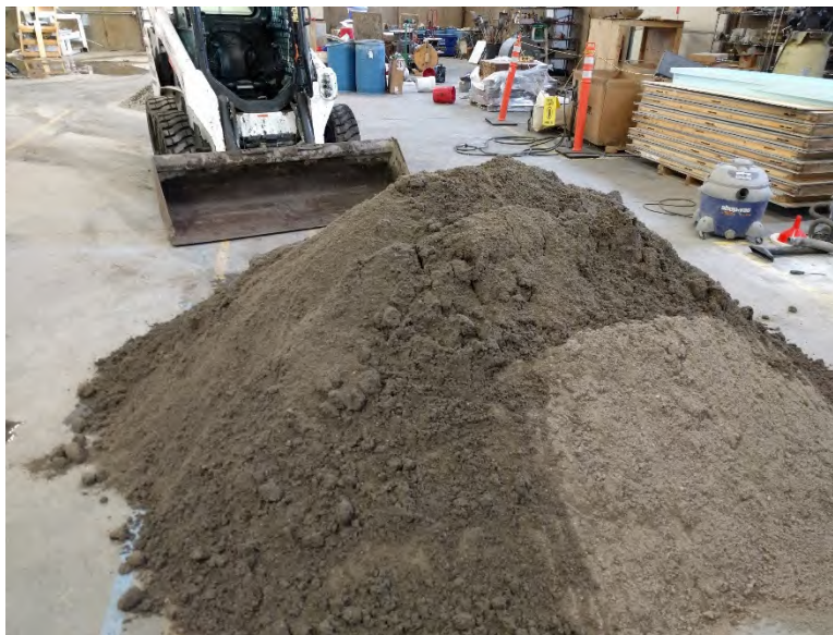
Figure 107 - Mixing fine aggregate and forming into pile.
