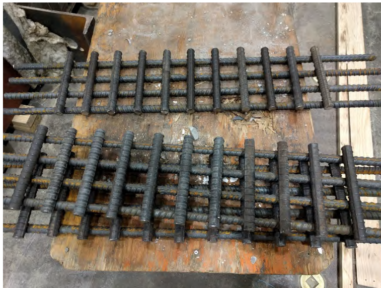
Figure 102 - Rebar cages ready to be welded to sample end plates.
