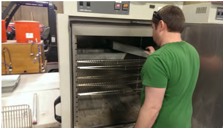
Figure 9 – Dana Schwartz of Fall Line placing washed material in drying oven.
