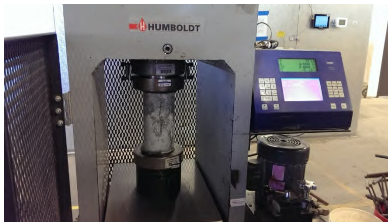
Figure 70 - Compression test apparatus
