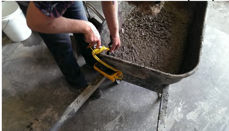
Figure 57 - Placing temperature probe
