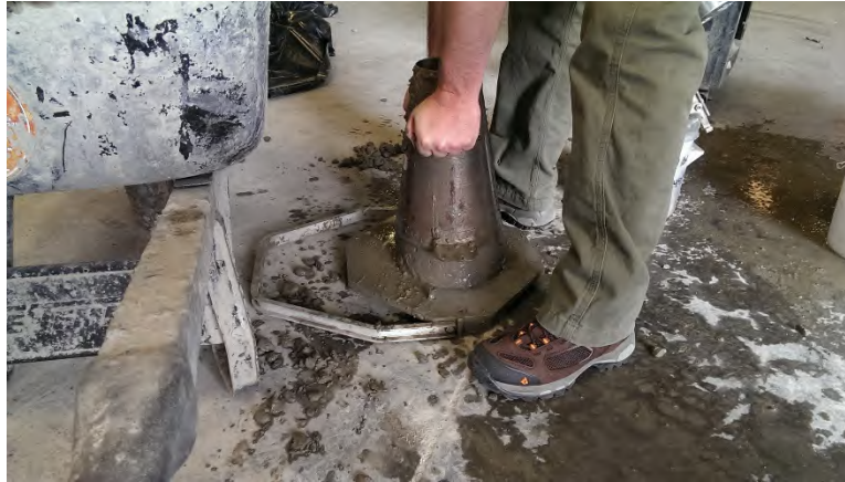
Figure 59 - The slump mold is lifted in one smooth motion.
