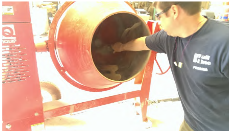
Figure 52 - Buttering the mixer
