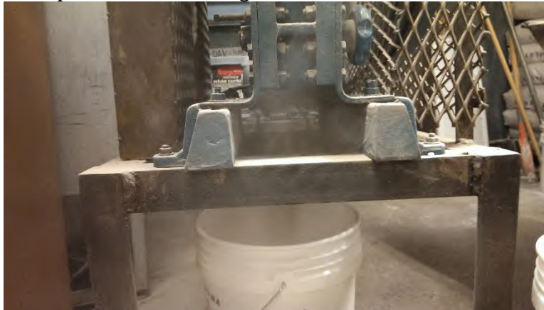
Figure 5 - Aggregate crusher in use at University of Colorado materials laboratory
