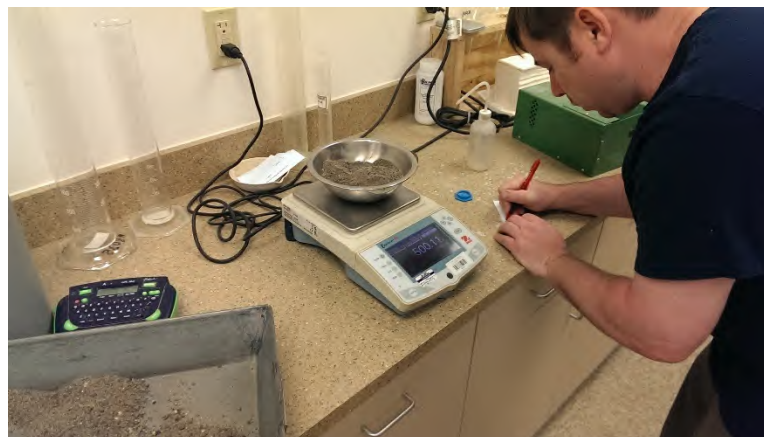
Figure 35 - A 500g sample of fine aggregate at SSD is weighed
