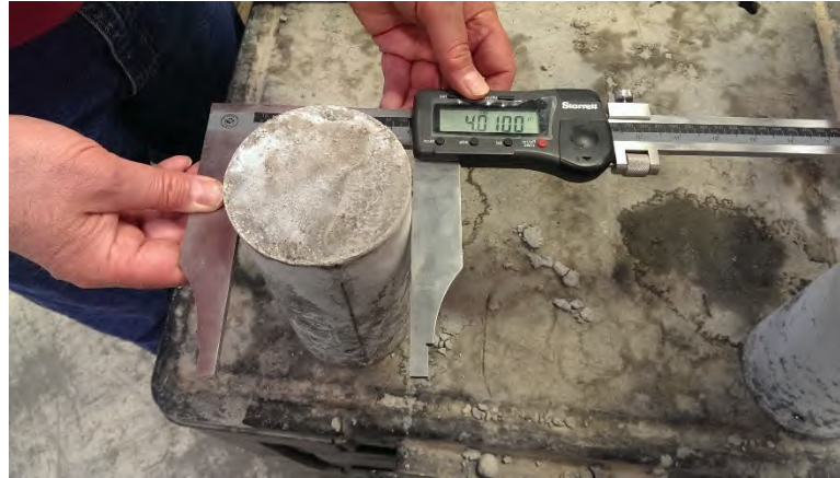
Figure 68 - Measuring cylinder diameter
