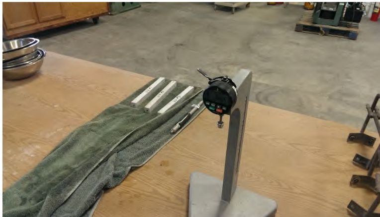
Figure 18 - Initial readings were taken before bars were placed in water bath.
