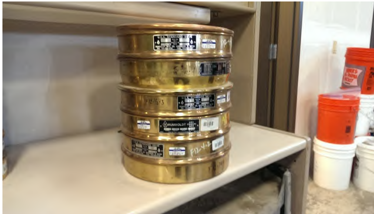
Figure 41 Sieve stack ready for coarse aggregate analysis
