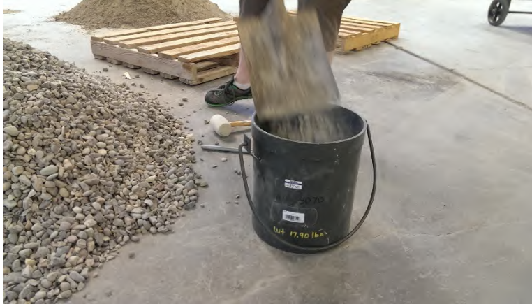
Figure 38 – Coarse aggregate is shoveled into the measure in three lifts.
