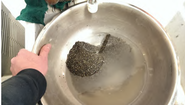
Figure 8 - Each grade was washed three to four times in tap water and decanted.
