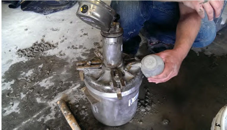
Figure 64 - A small quantity of water and isopropyl alcohol is added just until it begins to run out the weephole
