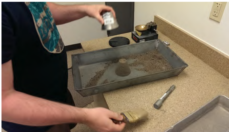
Figure 34 - Saturated surface-dry conditions are reached when sample slumps slightly when cone mold is removed. This sample does not slump and is still too wet.
