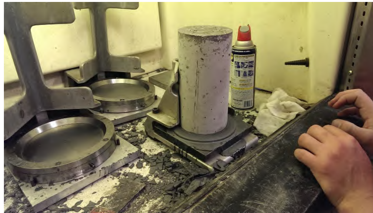
Figure 69 - Installing sulfur mortar end caps
