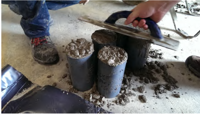
Figure 66 - Striking off cylinder molds
