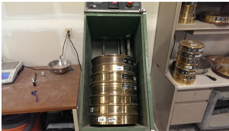
Figure 6 - Mechanical shaker with sieves at Fall Line laboratory
