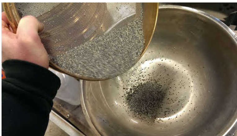
Figure 7 - The contents of each sieve were separated into steel bowls.
