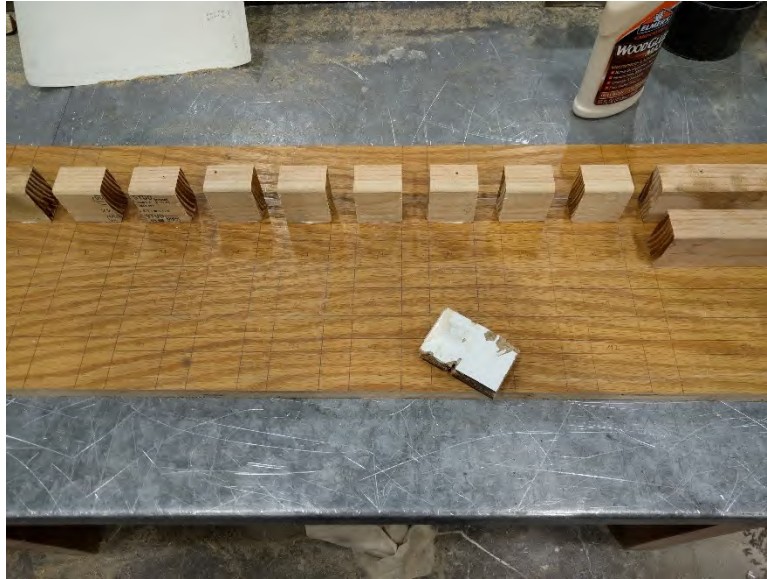
Figure 99 - Joining wooden blocks to jig base with wood glue and steel brad nails.
