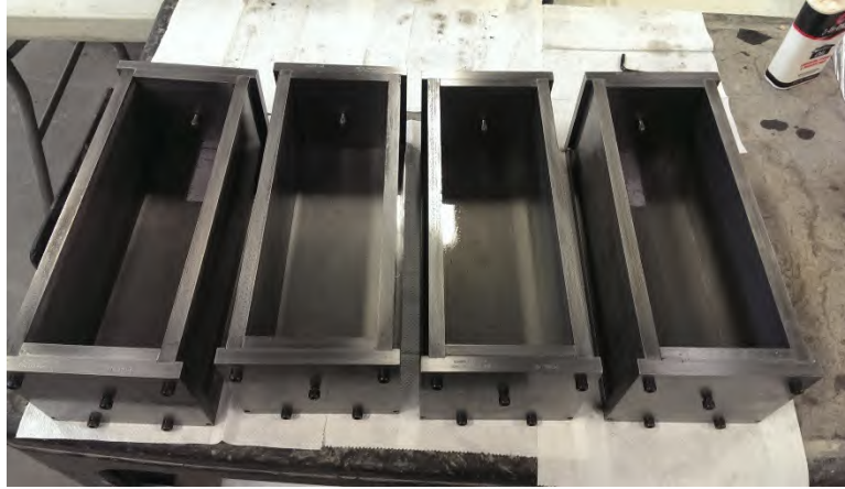
Figure 72 - 4-inch square prism molds ready for casting
