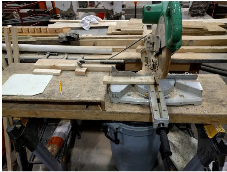
Figure 97 - Cutting wooden blocks for the welding jig.
