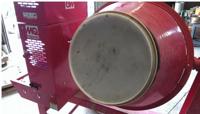
Figure 55 - Mixer is capped to prevent moisture loss during rest period
