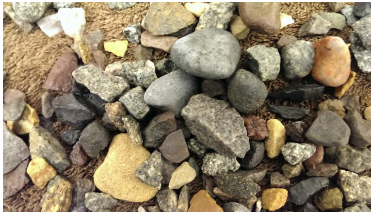
Figure 30 – Close up of coarse aggregate at saturated surface-dry condition
