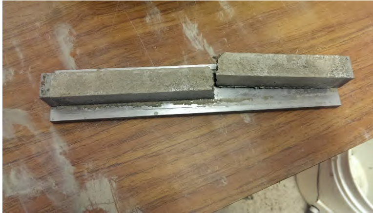
Figure 17 – This mortar bar broke during extraction
