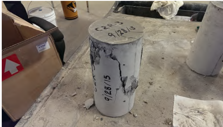
Figure 71 - Fractured cylinder after testing
