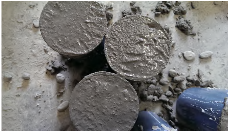
Figure 67 - Cylinders were allowed to rest 30 minutes before capping. Notice minimal bleeding.
