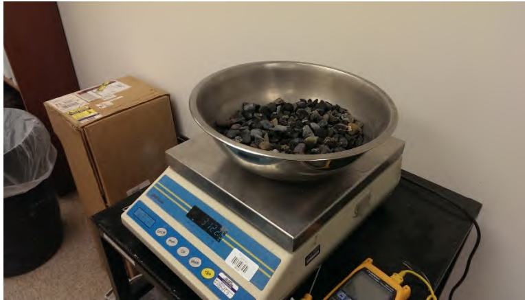
Figure 31 - Coarse aggregate at SSD is weighed
