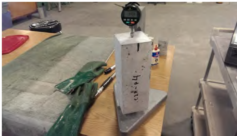
Figure 76 – Taking length comparometer readings of a concrete prism..
