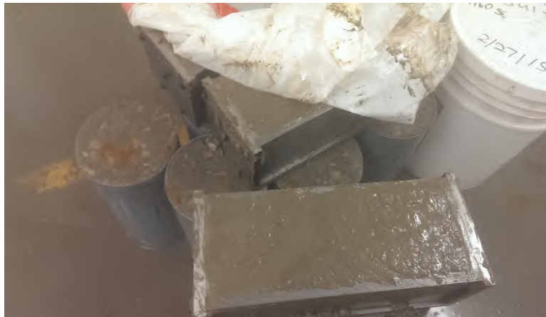
Figure 73 - 4 inch prisms are placed in fog room to cure 24 hours after casting.
