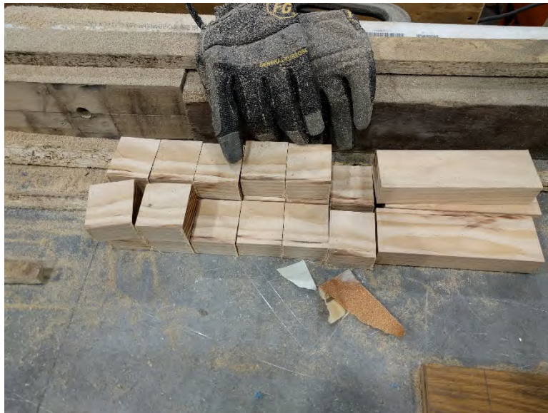
Figure 98 - Wooden blocks ready for installation in the jig.
