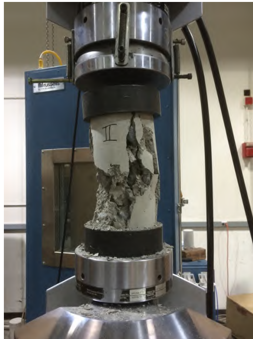
Figure 113 - Broken Cylinder in MTS Machine
