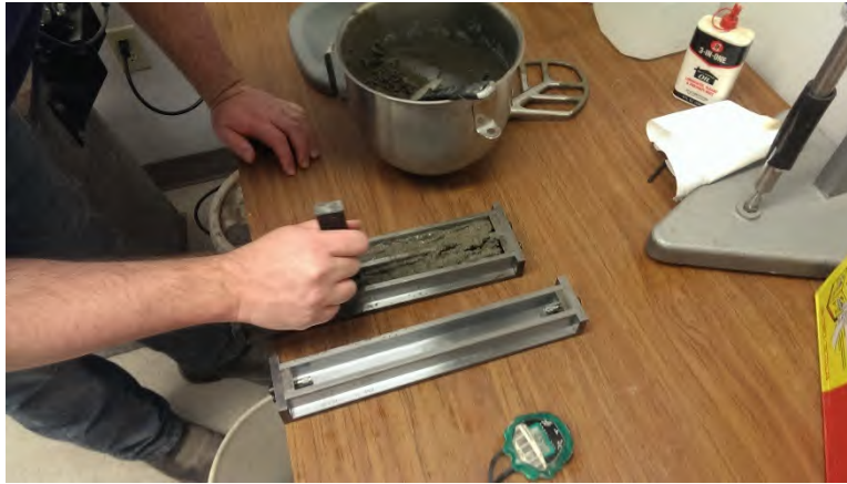
Figure 15 - Tamping mortar into molds
