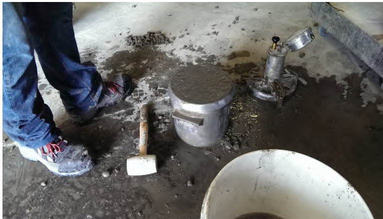
Figure 62 - After filling, the air meter bowl is struck off. Note the mallet used for tapping the bowl after each layer is rodded.
