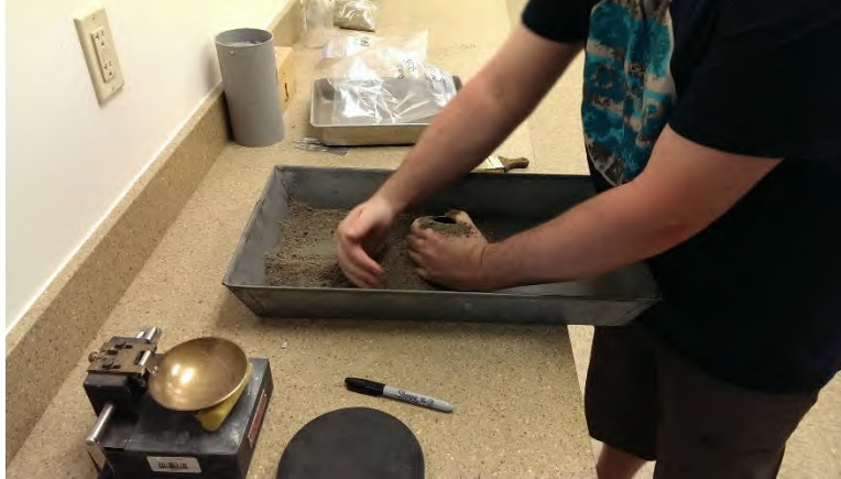
Figure 33 - Filling cone mold to check surface moisture of fine aggregate.
