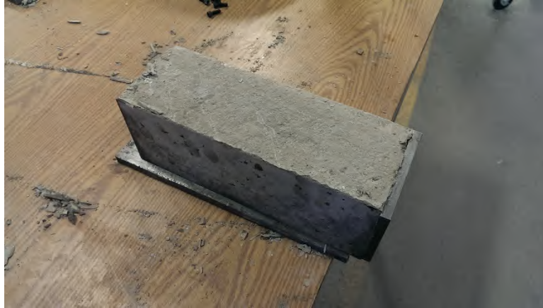
Figure 74 - Demolding a concrete prism.
