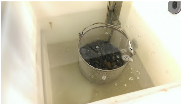
Figure 32 - Aggregate is immersed and weighed a second time. This apparatus allows the same scale to be used for both weighings.
