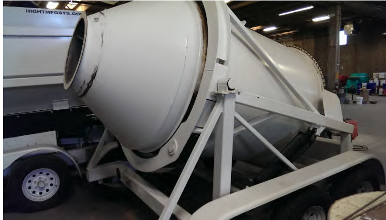
Figure 108 - The three-cubic yard mixer at Fall Line
