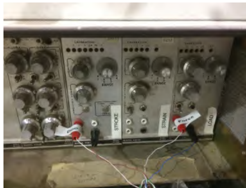
Figure 4.3: Force Displacement connections
