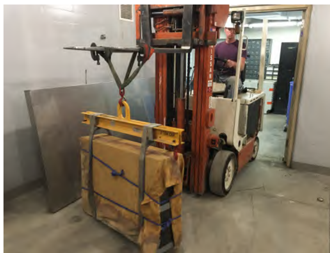
Figure 2.14: Placing shear specimen in fog room with forklift
