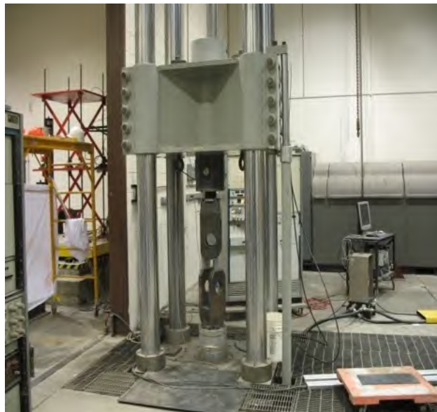
Figure A.1: MTS million-pound load frame
