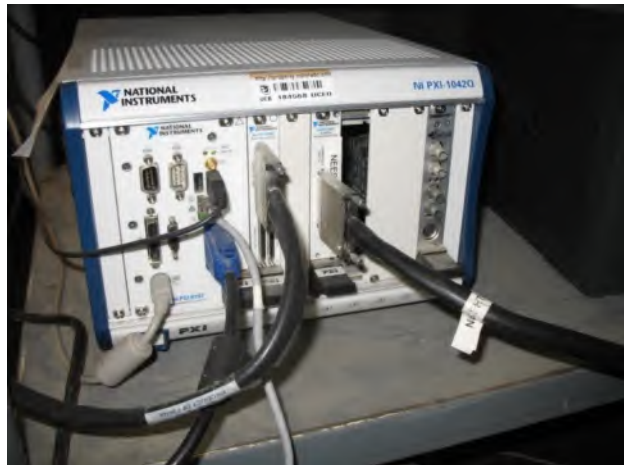
Figure A.3: National Instruments PXI-1042Q with embedded controller, data acquisition, and command
