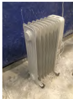
Figure 2.12: Electric space used to heat the fog room during heat installation
