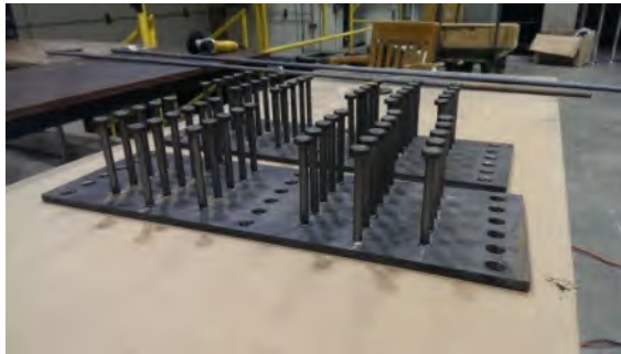
(c) Sample end plates with welded shear studs
