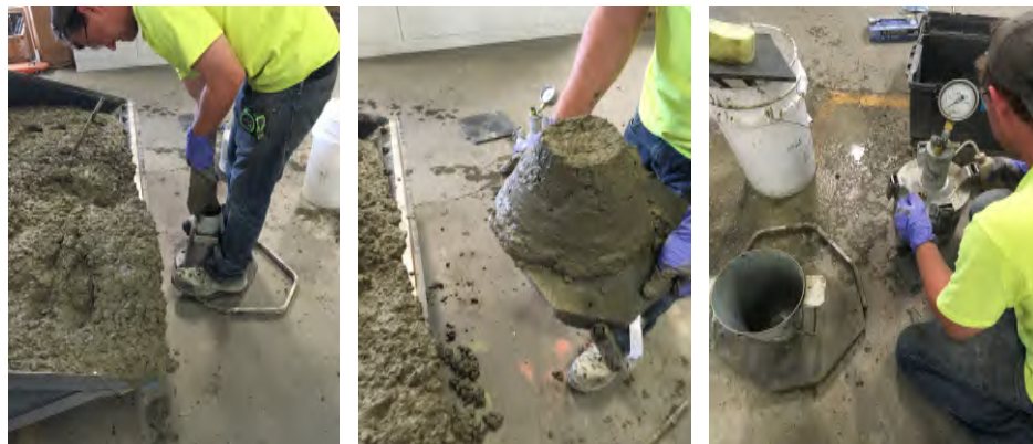
Figure 2.8: Slump and air content testing
