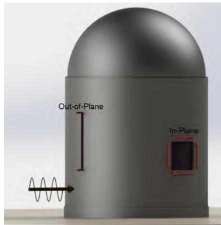
Fig. 36.13: in-plane and out-of-plane shear in a CEB [74]
