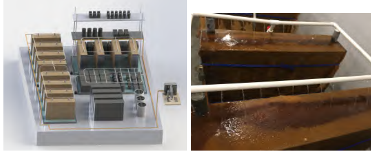
(a) Installation of reactive and non-reactive shear specimens, blocks, burlap-wrapped shear specimen prisms and cylinders in the fog room (b) Sprinkler system wetting the specimens
